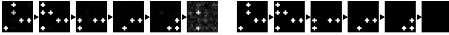
Fig. 6. Output of solving 4x4 LightsOut (left) and its binarized result (right). Although the goal state shows two blurred switches, they have low values (around 0.3) and disappear after rounding.
